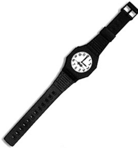
Figure 1. Actigraph (source: http://www.ambulatory-monitoring.com/products.html )
